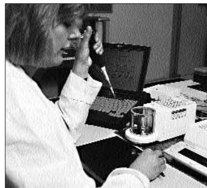
The Pipetman, an adjustable micropipette invented by two UW alumni, is a ubiquitous tool of biological research.
